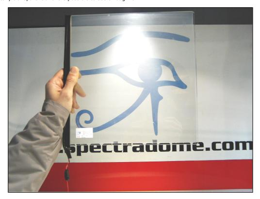
The second picture below shows the same previous LCD glass slab turned off: liquid crystal molecules are scattered in a way that deflects most of the ambient light and see-thorugh vision is impossible.
